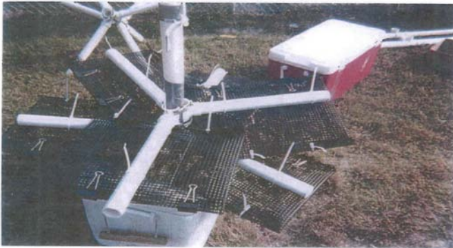
Figure 4-1 NASA LANGLEY RESEARCH FACILITY TABBS CREEK YEAR 2 BIOTA SURVEY/BIOMONITORING ASSESSMENT Photograph of Shellfish Biomonitoring Rack Used in Tabbs Creek.
