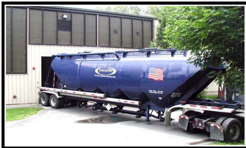
Delivery of carbon for groundwater treatment units
